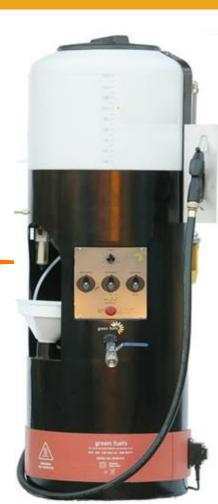
UCO to biodiesel small scale autonomous production unit
